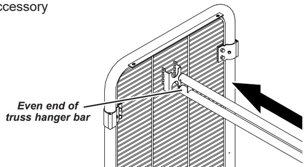
3. Lower the uneven end of the truss hanger bar into the upper pocket of the other accessory hanger bracket.
