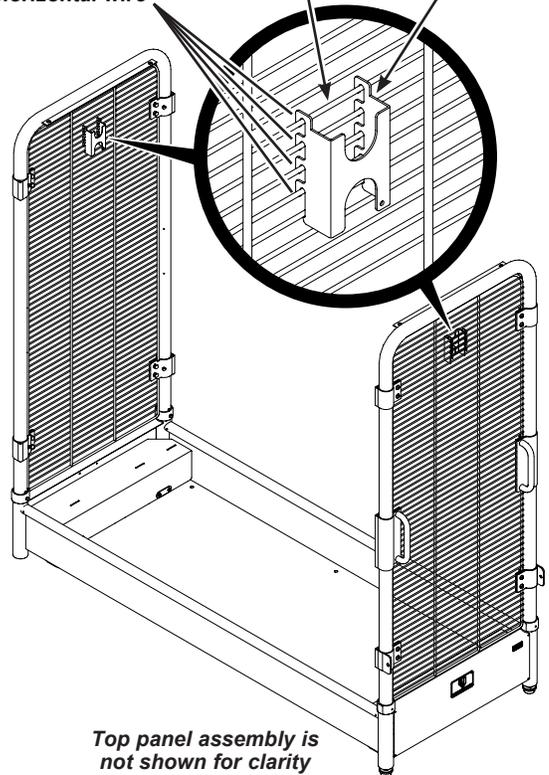
2. Insert the even end of the truss hanger bar into one accessory hanger bracket.
